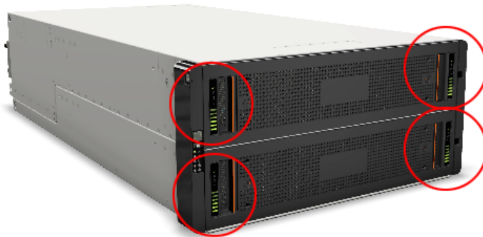
Figure 2-8 Drawer Sideplane Status panel locations
