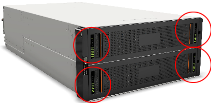
Figure 2-9 5U84 Primary Storage Shelf / 5U84 Expansion Storage Shelf Drawer Sideplane Status panel
